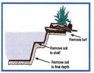
surface to install edging materials such as rocks, stones or railroad ties. The depth of the ledge should be sufficient to accommodate the edging materials and underlayment. The edging should extend about 1" to 1-1/2" above the surrounding terrain to prevent runoff from entering the pond. Also the edging will present a better appearance if it overhangs the water by 2 inches or so.
