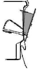
Use your fingers to hold the flange nut and a hand held screwdriver to tighten the screws. The serrations on the flange nut will grab the plastic
